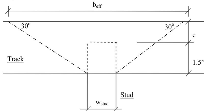
**Figure 2:** Stress distribution in track leg plate
