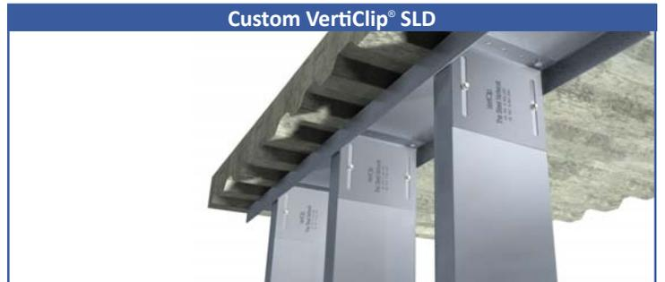
Connector for parallel wall studs. One stud rigidly attached to wall stud. The other stud accommodates vertical deflection of the primary structural frame.
