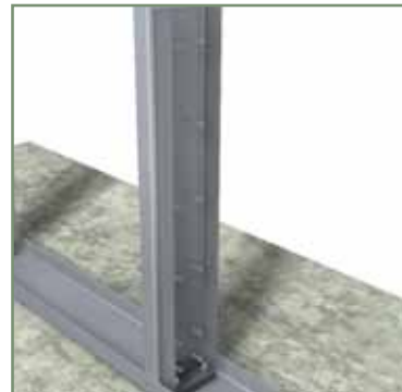
Attach MidWall™ 24" to the stud web with #12 screw fasteners through guide holes (fill all holes in the vertical MidWall™ leg).
