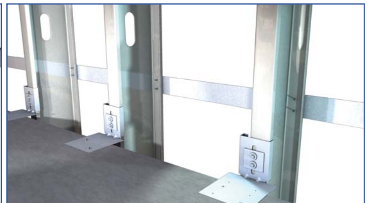
VertiClip SLF used with one flat strap bracing on the outer flange of studs to resist torsional effects.
