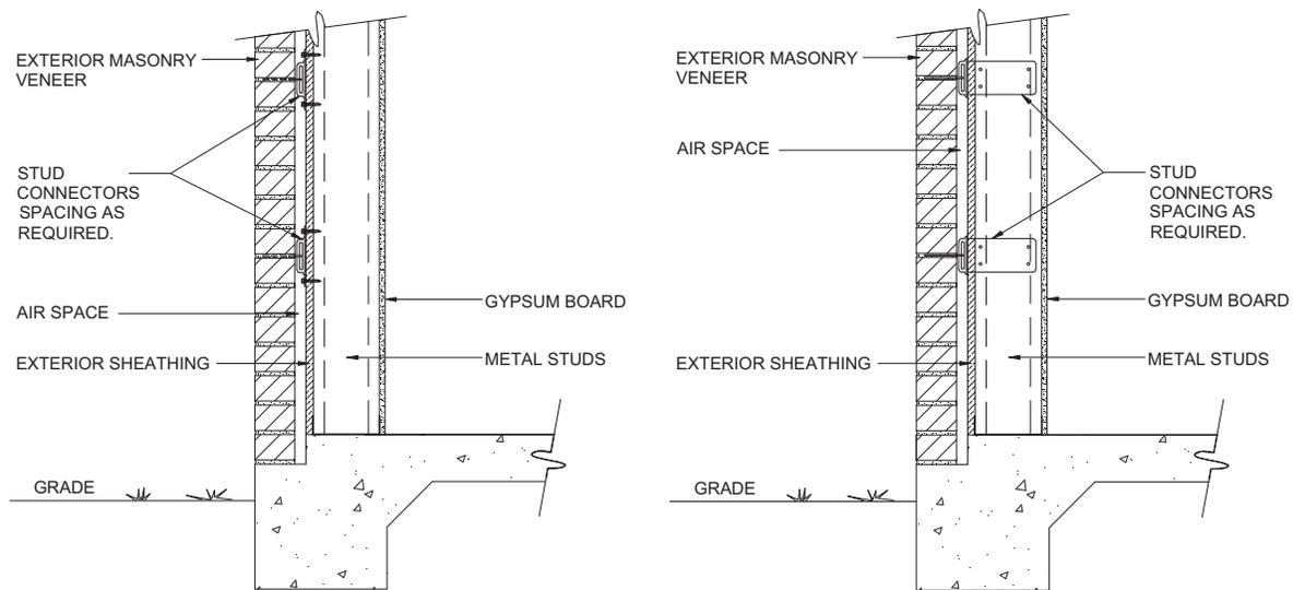
(a): Tie attached to stud Flange
