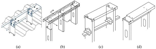
Figure 1: Vertical deflection connections at head-of-wall
