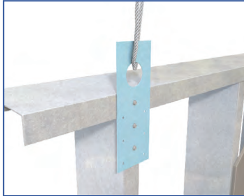
Attachment to Wall at Intermediate Stud
