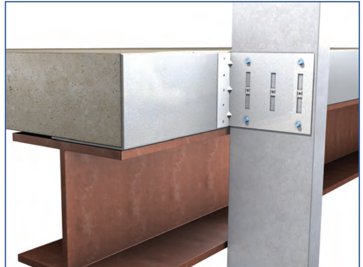
MasterClip® VLB used as Rigid Connection
