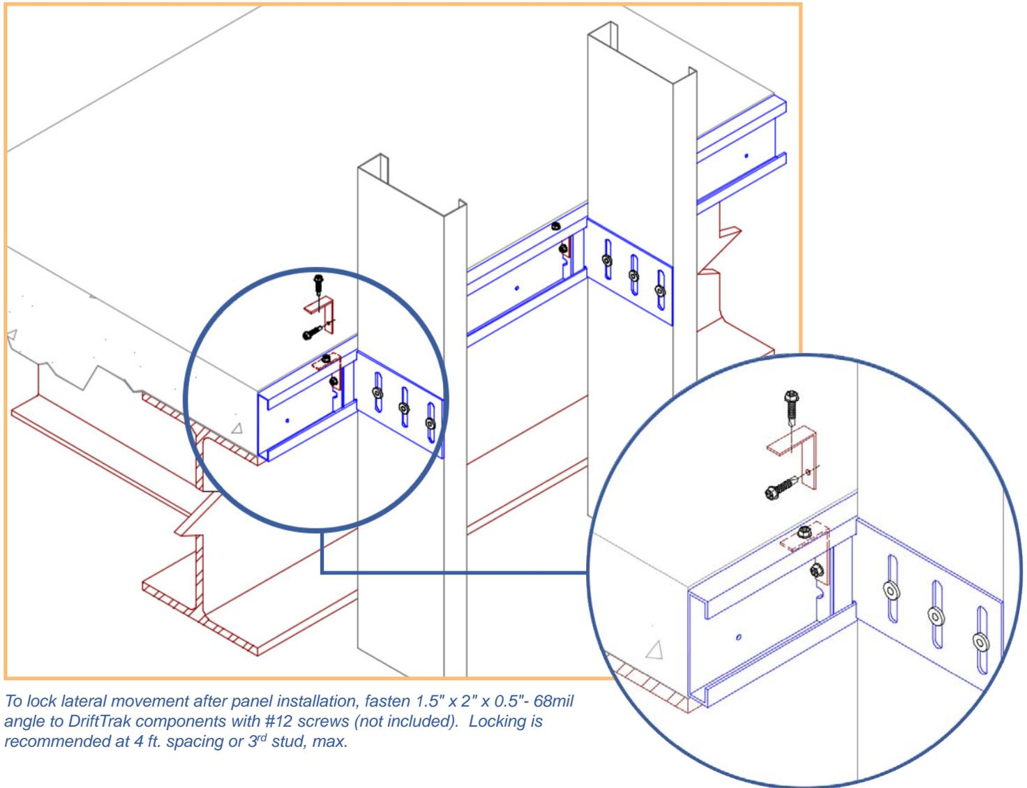
To lock lateral movement after panel installation, fasten 1.5" x 2" x 0.5"- 68mil angle to DriftTrak components with #12 screws (not included). Locking is recommended at 4 ft. spacing or 3<sup>rd</sup> stud, max.
