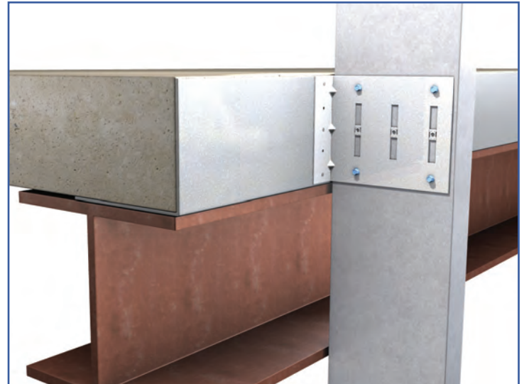
MasterClip® VLB used as Rigid Connection
