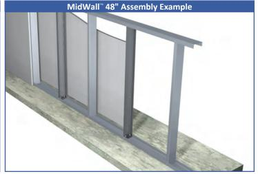
MidWall 48" is used in interior half walls equal to or more than 48" in height. Use one MidWall 48" as a substitute for a stud at MidWall connectors is 36" o.c.
