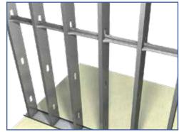
with standard "cee" studs, one screw is only needed every 3rd stud.\*
