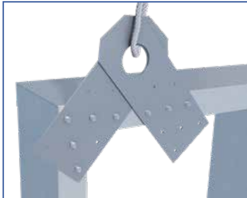
Double Attachment to Wall at End Stud
