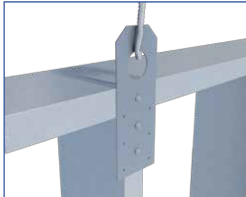
Attachment to Wall at Intermediate Stud
