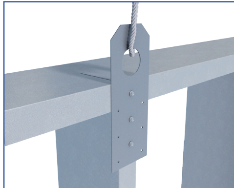
Attachment to Wall at Intermediate Stud
