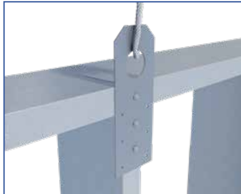
Attachment to Wall at Intermediate Stud
