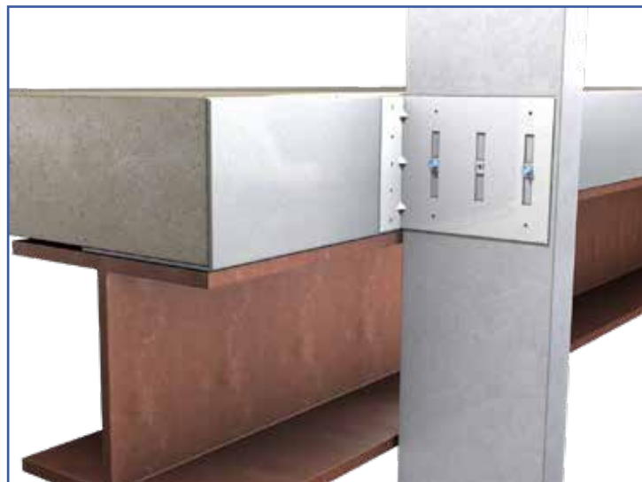
MasterClip® VLB used for Vertical Deflection
